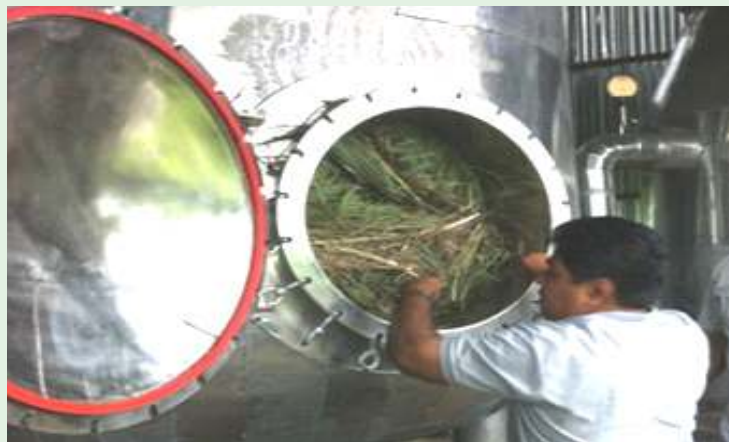
Biomass loading in distillation unit for essential oil extraction
