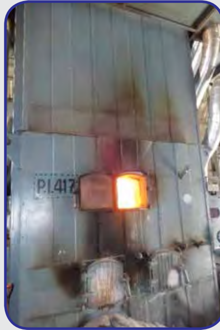
Burning of Rice Husk in Furnace
